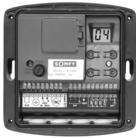
The **AXROLL** receiver is used to control a rolling garage door fitted with a 230V motor with built-in endstops using Keytis 2/4 RTS, Telis1/4 RTS, and Inis RT transmitters. Different safety and signaling systems can be connected to the **AXROLL** (sensor bar, photocells, flashlights, area lighting).
