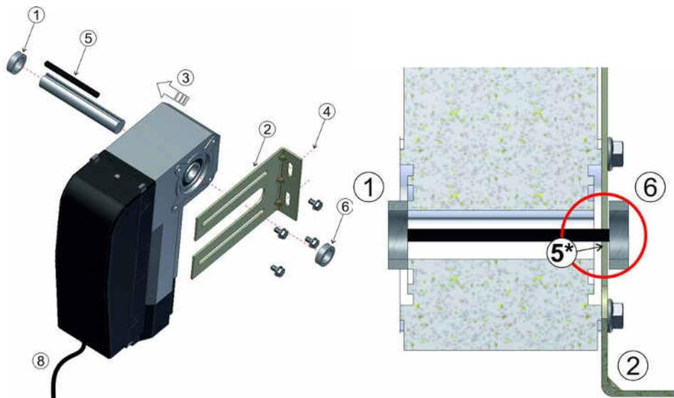
1. Attach the first stop ring to the shaft.
