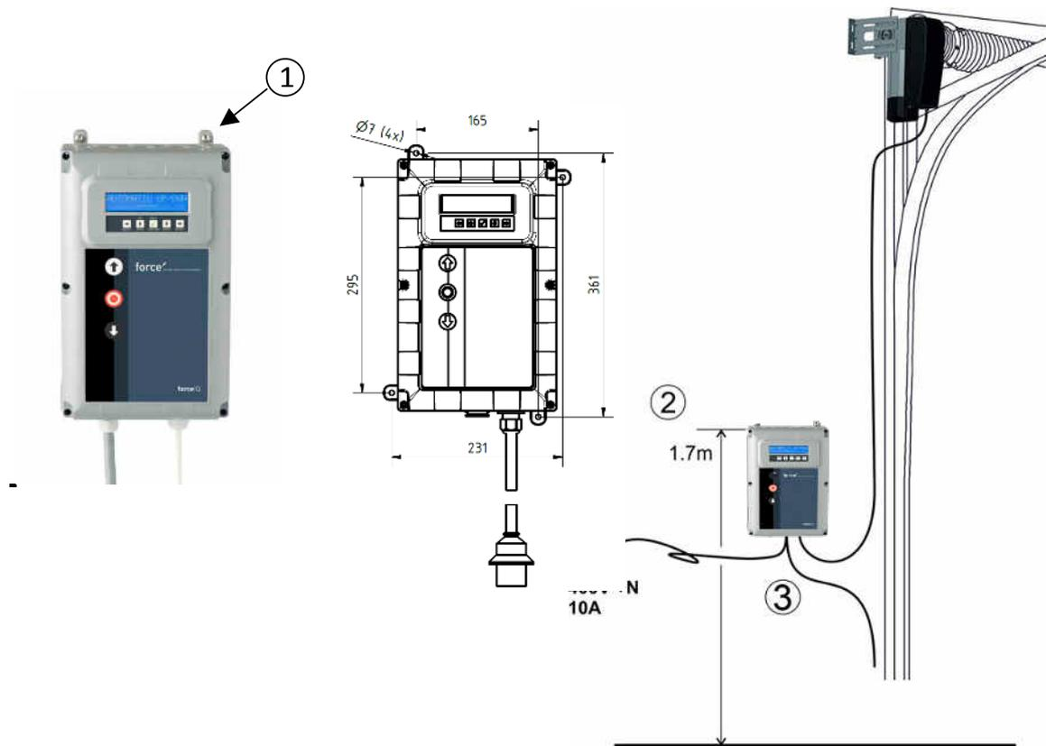
1. At the rear of the control unit you have to assemble 4 enclosure brackets before mounting it to the wall. Use the four small 5x12 screws.
