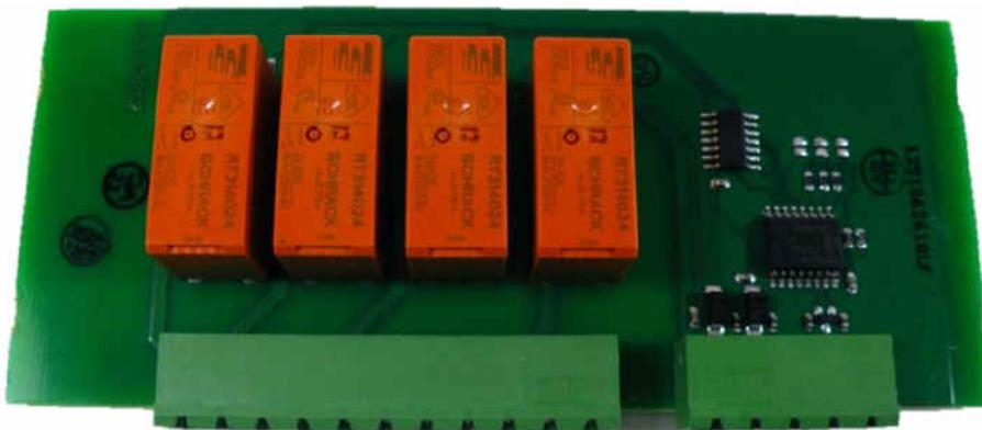
The Traffic light module has 4 integrated relays. The connection is at terminal KL22 in the ForceIQ. The detailed adjustments are described in the supplied manual and the wiring is shown in the electrical drawing. For more info and adjustments see 3.4.7 traffic lights page 20.
