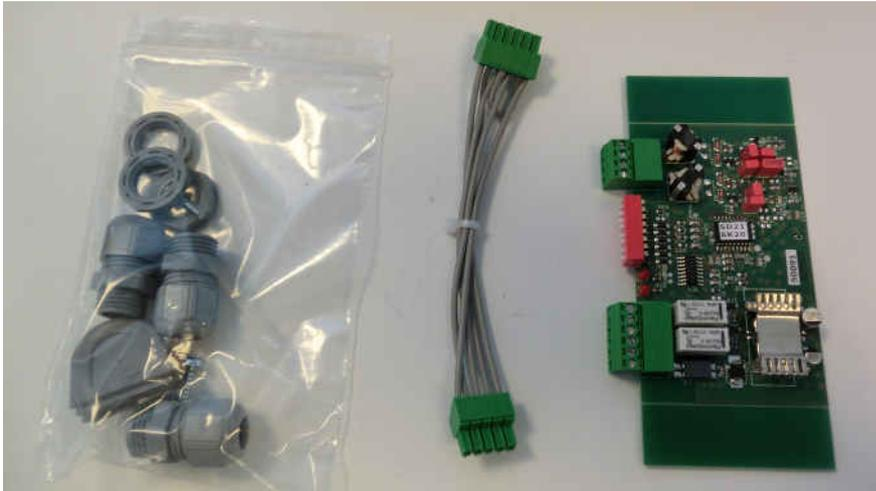
This is a double detector to connect 2 loops. The connection is at terminal KL23 in the ForceIQ.
