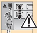
Permanently installed controls (such as push-buttons, switches etc.) have to be installed within sight of the door but well away from any moving parts at a height of at least 1.5 m. It is vital that they are installed out of the reach of children!
